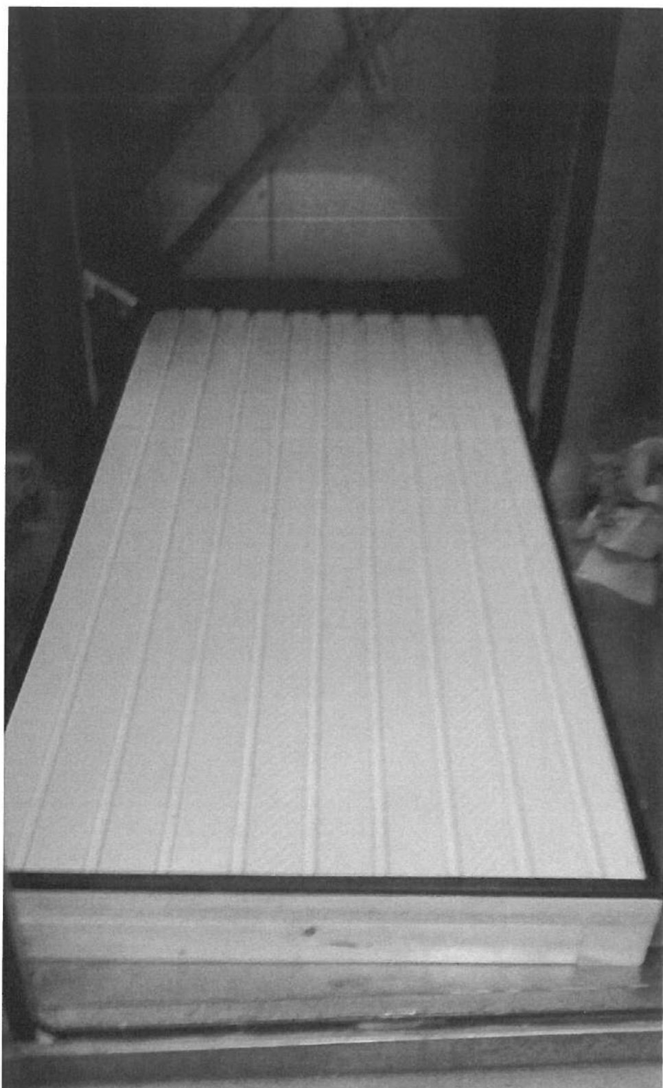
Phot. 1. View of the soffit tested in a climatic chamber (photo by LZE)
